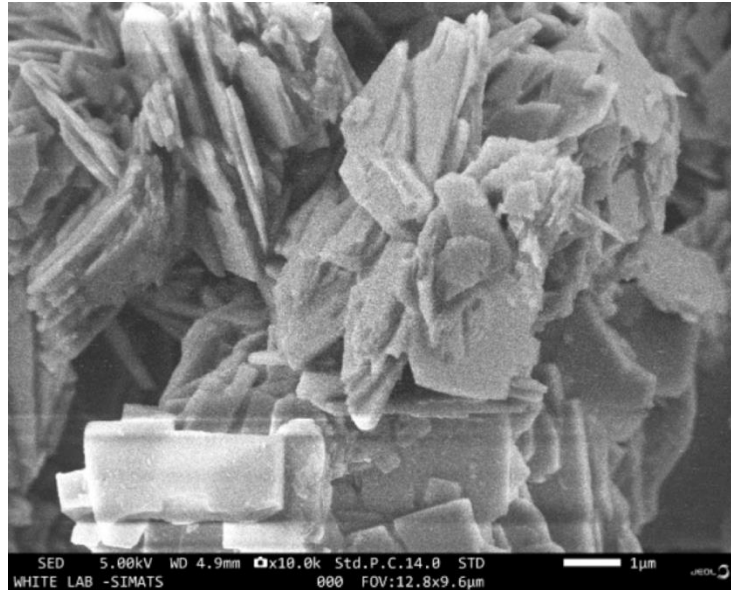
Figure 3: SEM analysis showing the morphology of the material synthesized, being coarse particle with crystalline structure and has the shape of stacked sheets.
