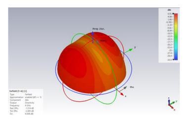
Figure 19, referred to as the Farfield\_axial ratio, illustrates the relationship between the main axis and minor axis of the polarization ellipse of an antenna operating at a frequency of 6 GHz. The degree to which an antenna is polarized in a circle is indicated by its axial ratio. The polarization of the wave emitted by a circularly polarized antenna varies with time.
