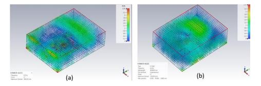
The directivity plots are displayed in Figure 16 (a) and (b) for both Excitation\_port1\_phi=0 and Excitation\_port1\_phi=90. The amount of energy that is transmitted in each direction can be shown using the directivity plot. Radiation angle is commonly shown on the x-axis and directivity on the y-axis of a polar plot. The directivity diagram for Excitation\_port1\_phi=0 indicates that the antenna's primary radiation is occurring
