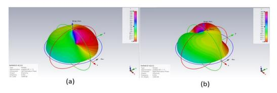
Figure 21 (a) and (b) depict the far-field radiation pattern of an antenna for left-handed (L) and right-handed (R) polarizations, respectively. The graphs indicate that the antenna has favorable directivity in the forward direction (theta=0 degrees) for both polarizations. The
