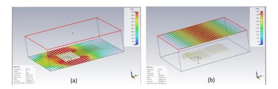
Figures 13 (a) and (b) show the magnetic field distribution at two different ports, namely Port 1 and Port 2, in the context of the passive 6G MIMO antenna design utilizing CST simulation software to achieve high gain. This illustration is helpful because it shows how the electromagnetic fields are spread and interact at various places, which affects the antenna system's overall performance and usefulness.
