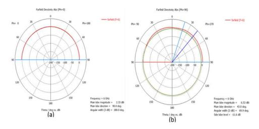
Figure 17 (a) and (b) are polar plots illustrating the antenna's far-field directivity at phi=0 and phi=90 degrees for excitation port 2's two possible excitation phases. For both excitation phases, the diagrams demonstrate that the antenna radiates a primary lobe in the forward direction (theta = 0 degrees). At 6 GHz, the magnitude of the main lobe is roughly 170 dB, and the angular extent of the main lobe is approximately 74.2 degrees.
