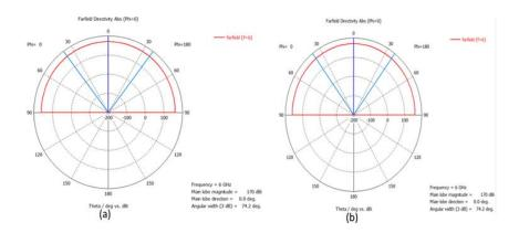
Figure 18 depicts the absolute directivity of an antenna in the far-field region, specifically at a frequency of 6 GHz. The plot illustrates that the antenna exhibits a peak directivity of 65.1 dBi when oriented in the forward direction (theta=0 degrees). As the angle theta increases, the directivity of the system diminishes and eventually reaches a minimum value of -27.4 dBi when the angle theta is equal to 180 degrees, corresponding to the reverse direction.
