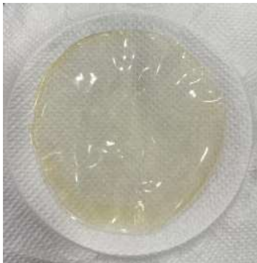
Figure 3: Showing the Zinc Oxide nanoparticle membrane after complete drying
