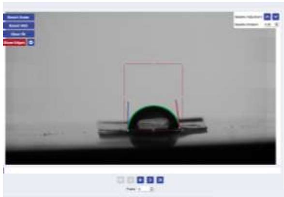
Figure 5: Contact angle of the test membrane =80.46°
