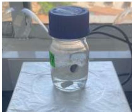
Figure 2: Preparation of Zinc Oxide nanoparticle membrane mixture placed on magnetic stirrer.
