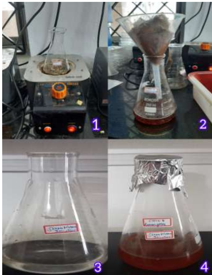
FIGURE 1: Preparation steps involved in clove and lemongrass extract-mediated synthesis of strontium nanoparticles.
