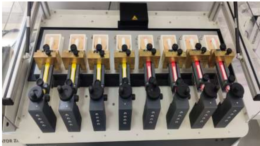
Figure 2: Composite resin samples subjected to brushing simulator
