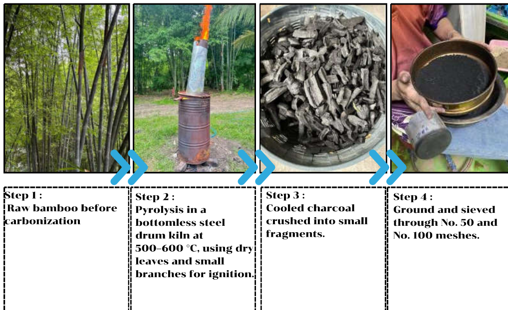
Figure 1: Preparation process of bamboo biochar
