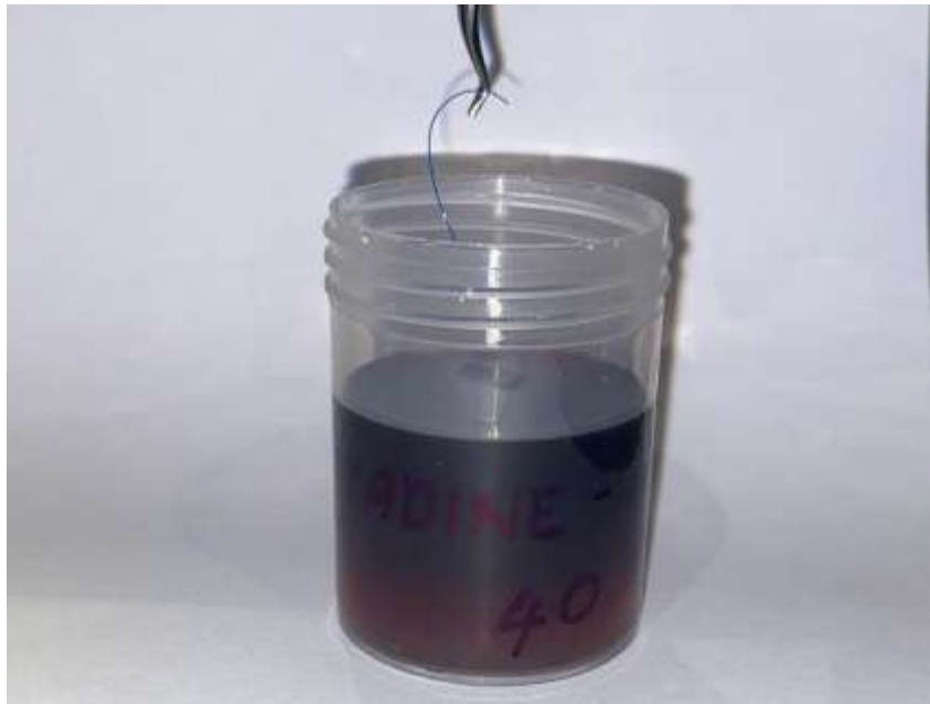
FIG 3: THE IMAGE ABOVE DEPICT THE SUTURE SAMPLE BEING IMMERSED IN BETADINE SOLUTION FOR 24 HOURS
