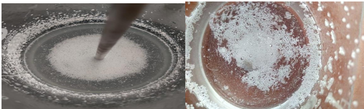
Fig. 1: Formed microballoons under mechanical stirrer
