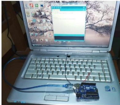
Figure 6: Computer-Arduino Board Interfacing
