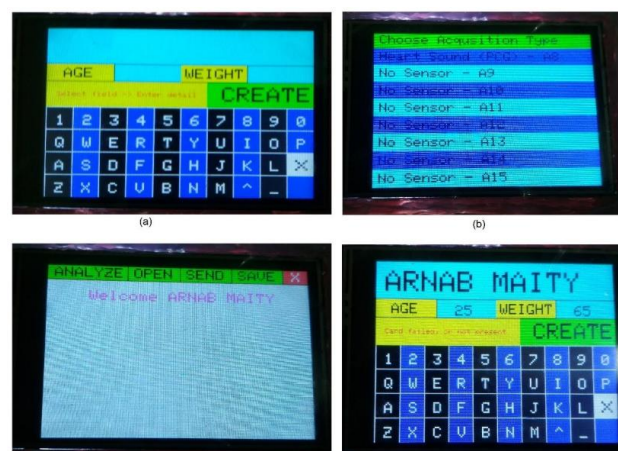
Figure 7: Different Windows of the Designed User Interface (a) Window for Patient Information (b) Window for Sensor Selection (c) Window for Functionality (d) Error Related to Memory Card Validation
