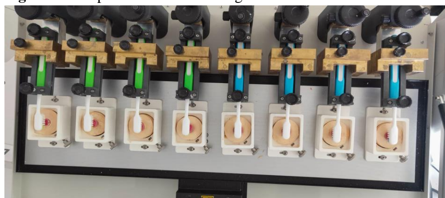
Figure 3: Brushing simulation done for 8 samples
