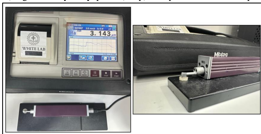
Figure 3: Represents the Stylus Profilometer-Mitutoyo SURFTEST SJ- 310 Surface Roughness Analyser used to obtain the values of surface roughness.
