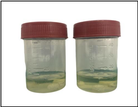
Figure 5: magnesium and strontium hydroxyapatite nanoparticles circular discs immersed in HiOra-K mouthwash for 24 hours.
