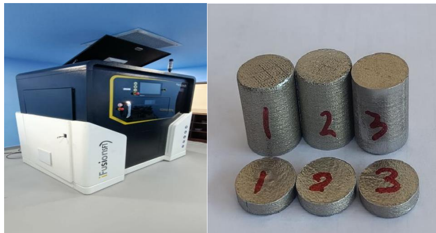
Fig 1. iFusion 150 metal fusion 3D printing machine and Fabricated Samples
