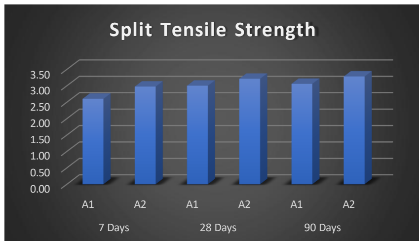
Split Tensile Strength Test Result (A1 VS A2) 7, 28 & 90 Days
