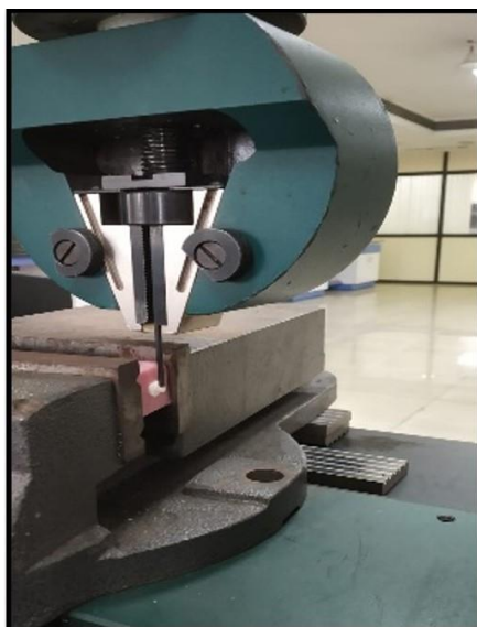
Figure 2: Testing of shear bond strength using universal testing machine
