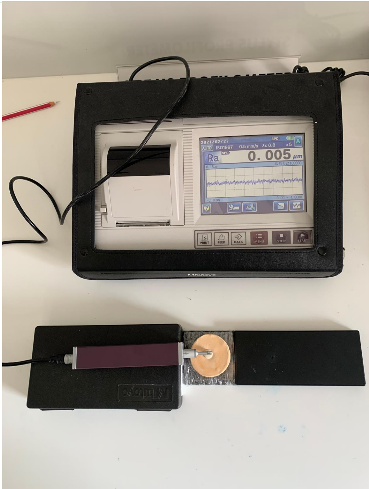
Figure 1: The image shows samples kept in a stylus profilometer for checking surface roughness pre and post brushing simulation.
