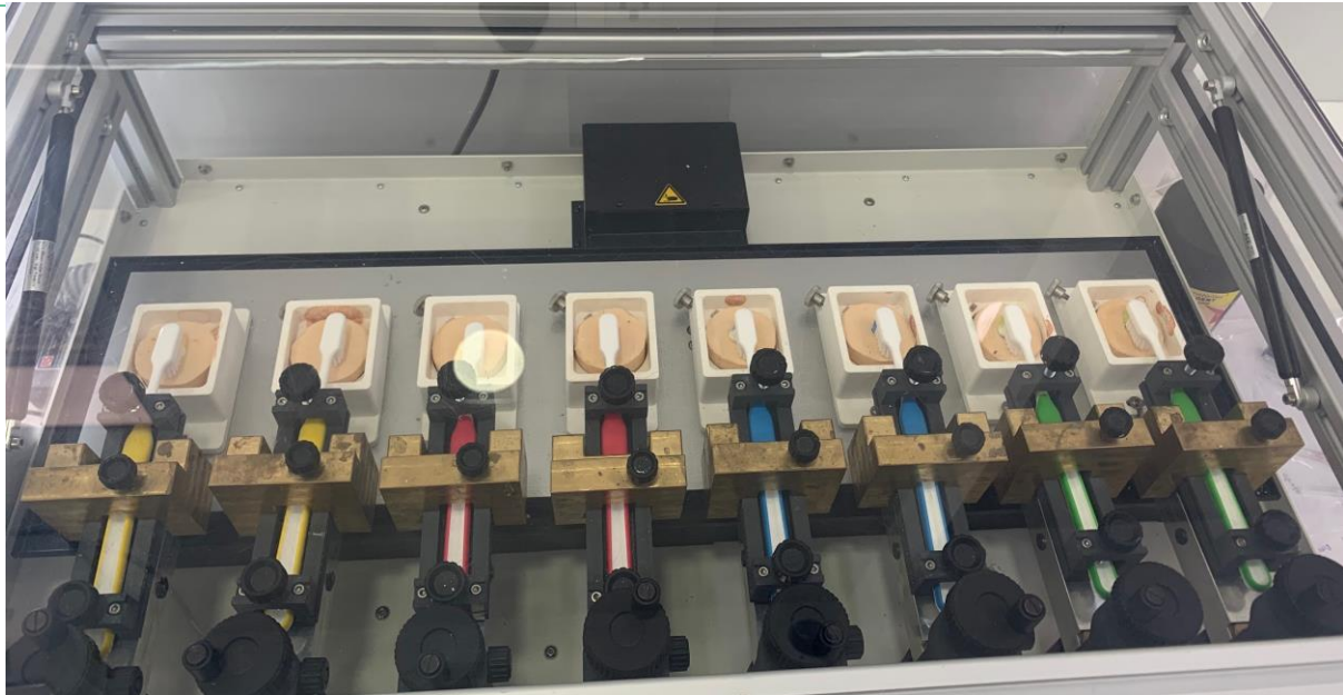
Figure 2: The image shows samples placed in the brushing simulator.
