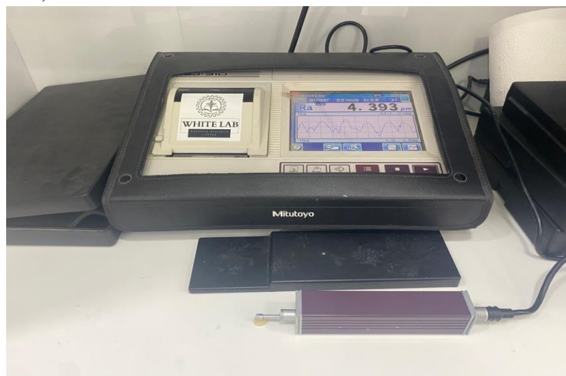
Fig 3: Represents the stylus profilometer used to obtain the values of surface roughness
