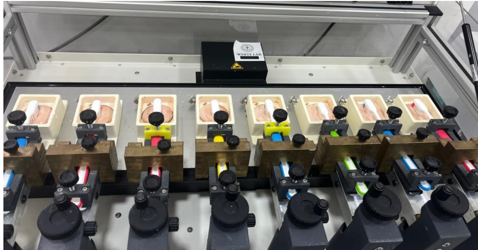
Fig 2: Samples were placed in the brushing simulation
