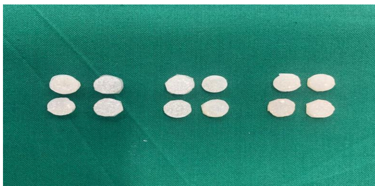
Figure 1: Samples from 3 different composite groups ( Group 1- Calcium composites, Group 2- Copper nanoparticles based composites and Group 3- Yttrium nanoparticles based composites )
