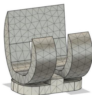
Fig 2.3. Meshed Model of Prosthetic Knee Joint
