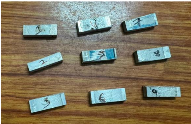
Figure 10 Photograph of fabricated Friction Stir welded hardness test specimens with addition of AgNO 3 Nano coated
