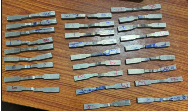
Figure 9 Photograph of fabricated Friction Stir welded tensile test specimens with addition of AgNO 3 Nano coated
