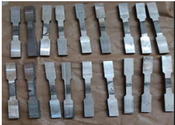
Figure 3 Photograph of fabricated Friction Stir welded tensile test specimens
