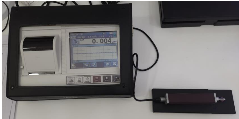
Figure 2: Represents the Stylus profilometer - Mitutoyo SJ 310, 2 \mu m tip/60°angle, device was moved physically on the surface of the light cure resin disc material to obtain the values of surface roughness
