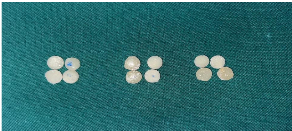
Figure1 :samples from 3 different composite groups (group1-Conventional composites, group2-magnesium based composites, group 3-strontium based composites)
