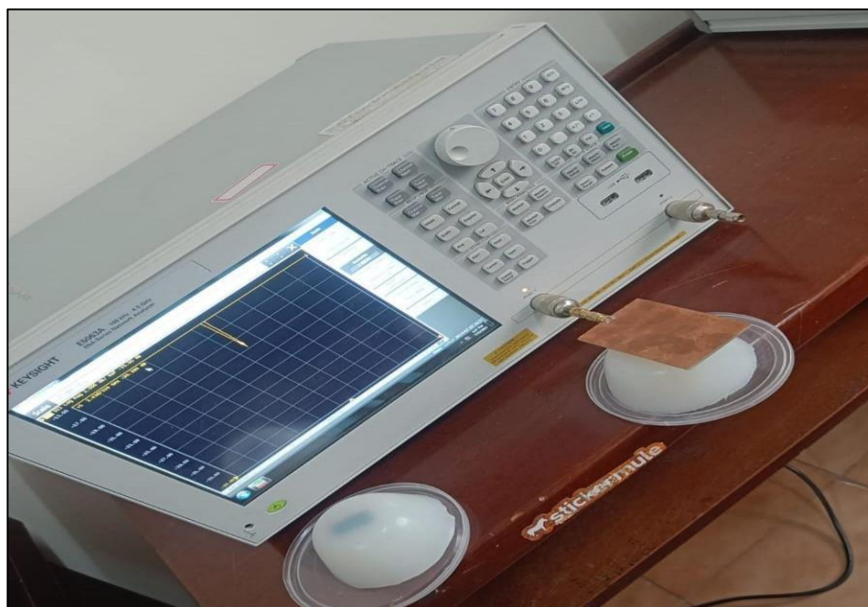
Fig 21. Testing of Fabricated antenna using VNA
