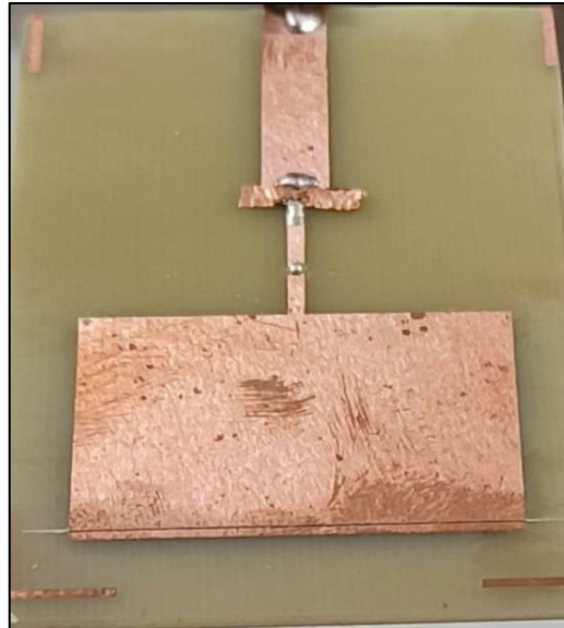
Fig 10. Fabricated prototype front view of proposed antenna
