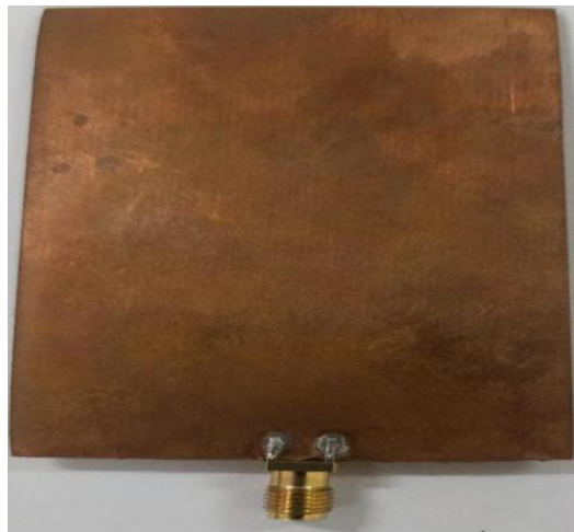
Fig 11. Fabricated prototype back view of proposed antenna
