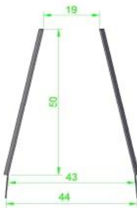
Fig. 2.2 Schematic view of Ridger (Dimensions in cm)
