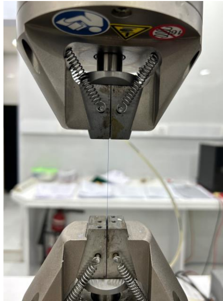
Figure 1: The above picture indicates the measurement of tensile strength polypropylene suture material using Universal Testing Machine.
